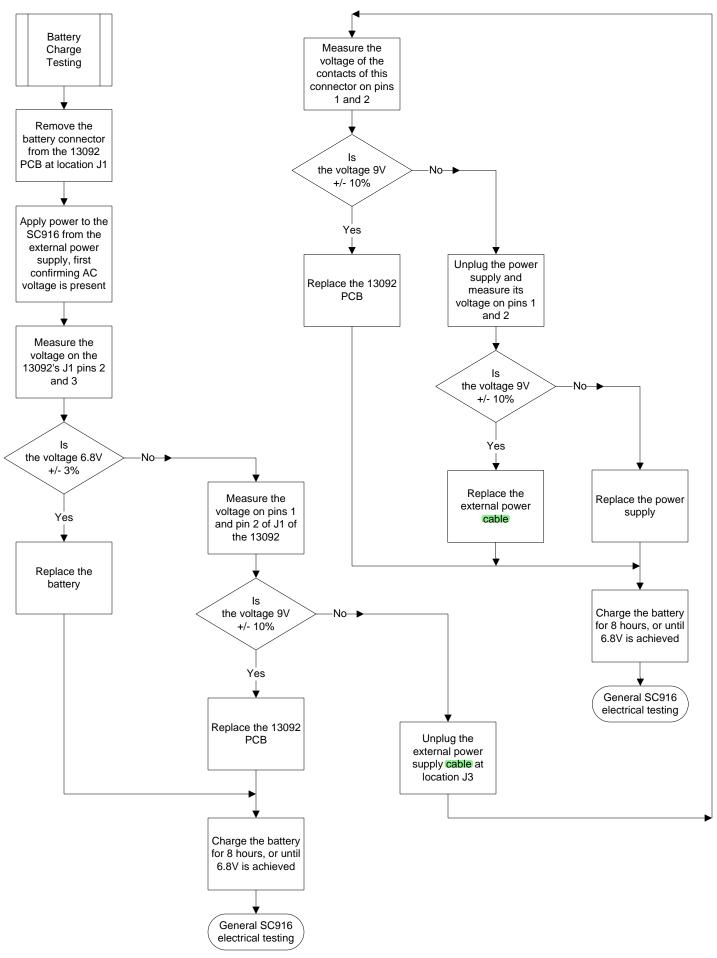
Due to requiring many pieces of test equipment, this procedure does not test the complete functionality of the charger but rather its final "float" state. If the battery voltage is less than 3V, no more than 50mA is applied. From 3V to 6.8V current control applies nearly .5A until voltage control or float state is entered.
