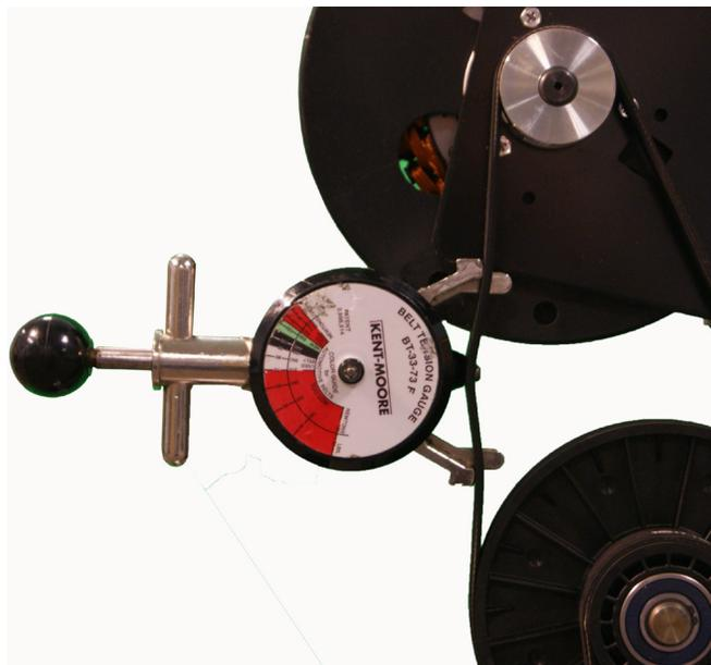
12 The belt gauge should read approximately  $90 \pm 10$  lbs. If the belt tension is significantly high or low the belt tension may be adjusted by loosening the generator mounting bolts.
