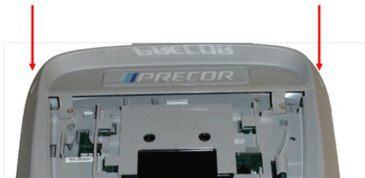
11 Remove the 6 screws that fasten the rear cover from the console and remove.
