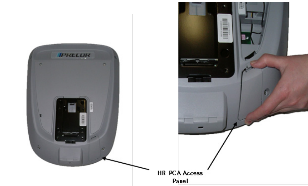
Figure 13: HR PCA Access Panel
