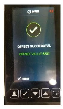
Once the calculation is finished, the screen will respond with "Offset successful" at this time use the "check mark" to select "finish" and then exit the setup screen and test the bike. If the offset is unsuccessful, the bike may need a mechanical repair or adjustment.
