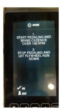
Once you select this option, the instructions will come up on the screen. Use the "check mark" to select "OK" and start pedaling. The RPM will appear on the screen. Pedal until the RPM reaches over 10, then let the bike coast to a stop from there:
