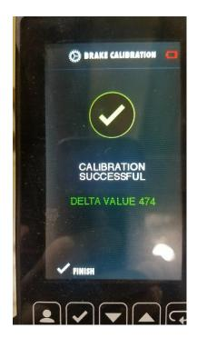
The screen should read "Calibration successful" if it does not the resistance may need a mechanical adjustment.
