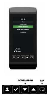
Step 1 – enter the setup/diagnostic mode by holding down the "down arrow" and "lap" keys from the main screen.
