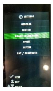
Using the "down arrow" scroll to the "BRAKE CALIBRATION" option, and use the "check mark" to select "next"
