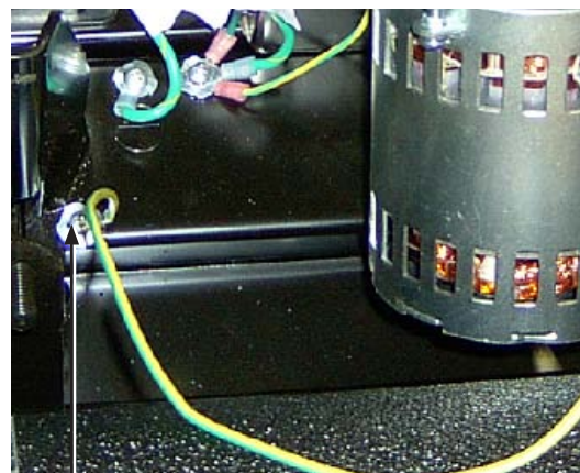
Ground Screw (12-18 in-lbs) [1.3-2 N-m]
