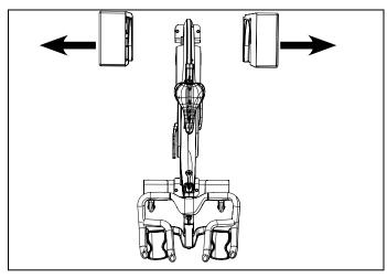
6.3 Carefully remove the tape from the frame before the stabilzer is mounted.
