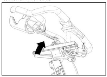
6 mm ball hex socket Torque: 30 Nm
