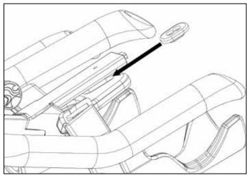
8.2 Slide the bike computer onto the computer bracket.
