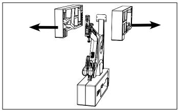
1.9 Carefully remove the tape from the frame before the stabilzer is mounted.
