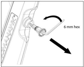
**Caution:** Never remove the safety pin before the handlebar has been mounted on the bike.
