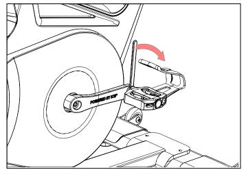
Tighten the pedal marked "L" on the left crank arm by turning in the clockwise direction to 55 N.
