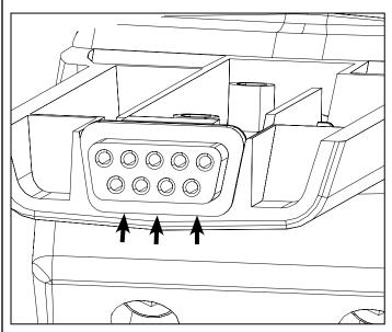
Position the smaller side of the connector to the lower side of the bracket.
