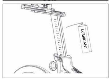
Check height adjustment and pop pin function of the handlebar and seat height adjustment.
