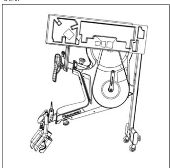
6.2 Take the Styrofoam off the bike and be sure to remove all parts taped inside.
