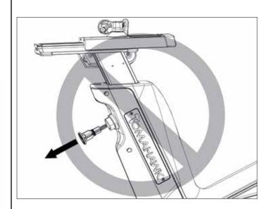
THE VERTICAL HANDLEBAR STEM OF THE INDOOR CYCLE IS SPRING LOADED AND WILL EXTEND QUICKLY UNLESS THE HANDLEBAR IS MOUNTED ONTO THE STEM. EXTENSION OF THE STEM WITHOUT THE MOUNTED HANDLEBAR MAY CAUSE INJURY OR/AND DAMAGE TO THE INDOOR CYCLE.
