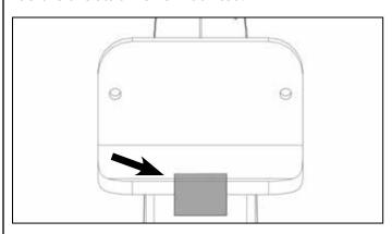
6.4 Fasten the rear Stabilizer and mount the caps to the top of the frame
