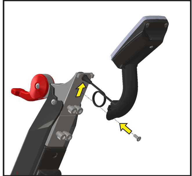
Figure 12. Attach the Computer to the Handlebar Tube
