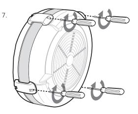
3. Check screws for tightness, including those used for assembly.
