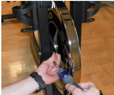
6. Install the sensor, screw on the top and bottom screw (Fig. 8).
