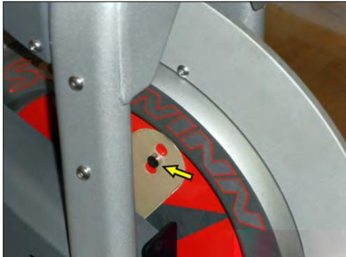
8. Turn flywheel to verify the light on the sensor lights up.
