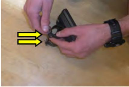
4. Wrap the loops around the handlebar. (Fig. 5 & Fig. 6). NOTE: If loops do not fit snugly around the handlebars, use the rubber shims to take up the slack.
