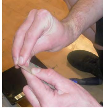
8. Place plastic piece so that the curve at the bottom sits against the axle hub (Fig. 10).
