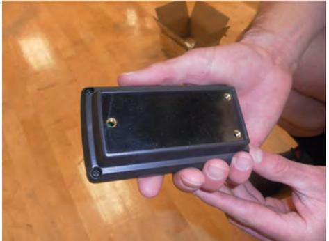
2. Place the 2-loop mount on the back of the computer and tighten the 3 screws to the computer (Fig. 3).
