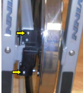
7. Peel off the adhesive patch that holds the magnet to the flywheel (Fig. 9). Place plastic piece so that the curve at the bottom sits against the axle hub (Fig. 10).
