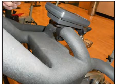
5. Install the sensor, screw on the bottom left screw (Fig. 7).
