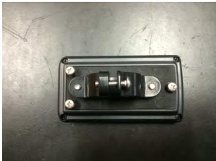
3. Unscrew screws that hold the loops together (Fig. 4).
