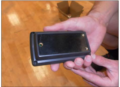
2. Tighten the 3 screws to the computer (Fig. 3).
