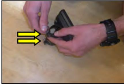
4. Insert clip on to the handlebar computer facing upwards (Fig. 5 & Fig. 6). NOTE: If loops do not fit snugly around bars, use the rubber shims to take up the slack.
