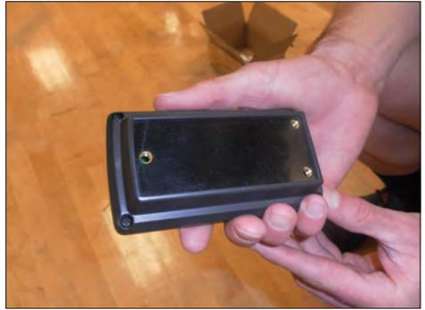
2. Place the one-ring mount on the back of the computer. Insert and tighten the three mount screws (Fig. 3). Remove the screw that holds the loop together (Fig. 4)
