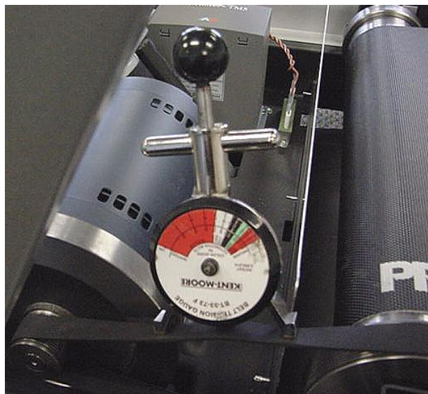
Diagram 8.2.1 - Drive Belt Tension Gauge
